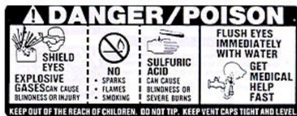
Lead-acid batteries contain hydrogen-oxygen gases that can be explosive and sulfuric acid that can cause severe burns.
