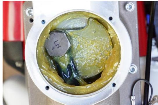
Figure 3 Crank area with sufficient grease. Colour is yellow prior to use as above, and will tend to brown with age and use
